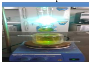
Figure.1. Main parts of the photocatalytic cell used in Photocatalytic degradation of Safranin-O dye
